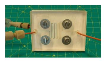
Micro reactor used for testing the CO<sub>2</sub>-permeability of membranes (source: University of Twente, NL)
