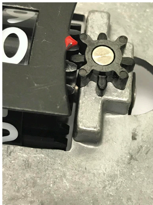
Figure 34: Pinion counter wheel alignment on whole numbers
