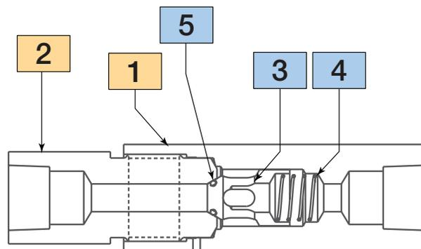
Do Not use check valve body (1) to tighten gland nut (2) into mating connection. Seal damage will occur.
