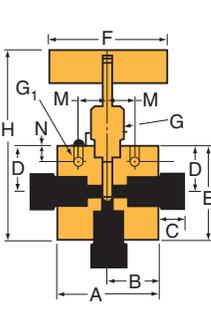
G - Packing Gland mounting hole drill size • G1 - Bracket mounting hole size • H\* - Dimension is with stem in closed position
