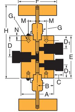
G - Packing Gland mounting hole drill size • G1 - Bracket mounting hole size • H\* - Dimension is with stem in closed position
