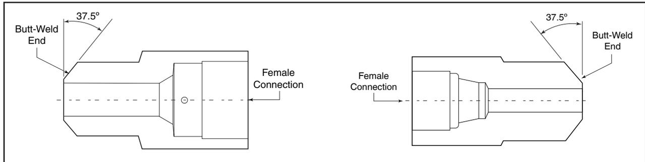
Note: Standard Butt-weld adapters made from 316 SS.
