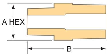
The diagram shows a side view of a pipe hex reducer nipple. Dimension 'A HEX' is indicated by a vertical double-headed arrow on the left, representing the hexagonal width. Dimension 'B' is indicated by a horizontal double-headed arrow at the bottom, representing the length of the nipple.
