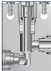
In some applications, more precise flow control is required than is possible with a Vee stem. For these cases, Autoclave offers a non-rotating, two-piece regulating stem which can be used for both control and shut-off. While it is not as precise as the control associated with the MicroMetering stem, especially with smaller flows, it does offer substantially better control than the Vee stem.
