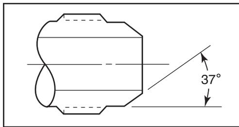
JIC connections consist of a 37° angle.
