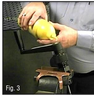
6. Apply cutting oil through the lubricant opening in the end of the cutter holder or directly through the housing window (Fig. 3). A medium weight high sulphur content cutting fluid is recommended. Use the cutting oil freely during the coning operation.
