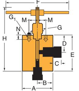
G - Packing Gland mounting hole drill size • G1 - Bracket mounting hole size • H\* - Dimension is with stem in closed position
