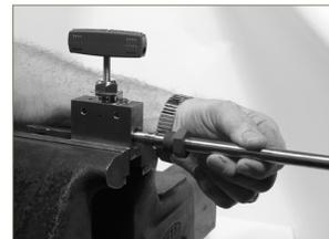
**Step 3.** Turn gland until "finger-tight", THEN, TIGHTEN GLAND UNTIL SLEEVE BEGINS TO GRIP TUBING by using wrench, turning until you feel increased resistance. This is what we call "Wrench-Tight". (this differs from standard compression fitting installation)
