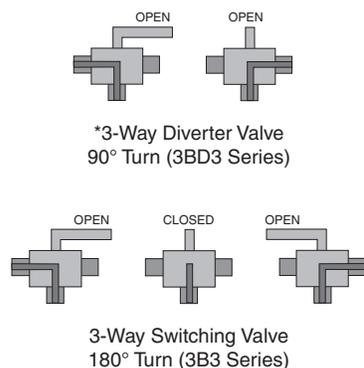
\*The Diverter Valve design permits inlet flow through the bottom port. Outlet flow may be diverted to either valve side port with only a 90° turn.
