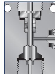
Replaceable seat option is only available with Right-Angle Style body. Replaceable seat is supplied as standard with an additional seat - rotate to use second side. Can be used with either stem type. Options include Stellite material or N-Dura coating to increase service life.
