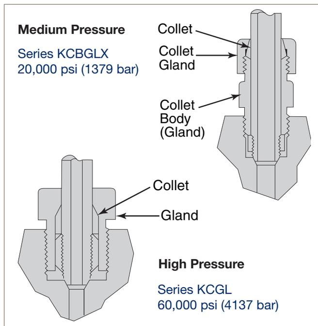
**Note: Always use a back-up wrench on collet body to prevent over tightening of collet body into connection.**
