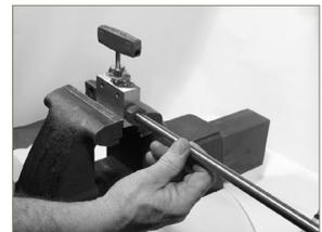
**Step 4.** From this "Wrench Tight" position, note starting position of wrench. Tighten gland approximately 1-1/4 turns for the SW and 1/16" & 1/8" W connections. When installing Male Adapter (preformed ferrule tip) fitting, - only 1/8 turn is necessary.
