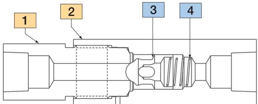
Do Not use check valve body (1) to tighten gland nut (2) into mating connection. Seal damage will occur.
