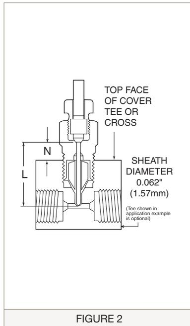
**Note:** All thermocouples are furnished complete with 1/4" Medium or High Pressure connection adapter to match tubing size selected. Union Tee or Cross sold separately.
