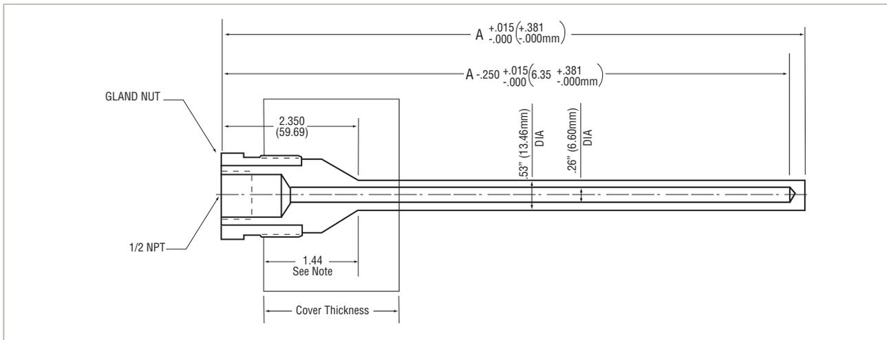
**Note:** Thermowells fit Autoclave's 1" medium pressure connection. (SF1000-CX). 1" connection insertion length is 1.44" (36.76).
