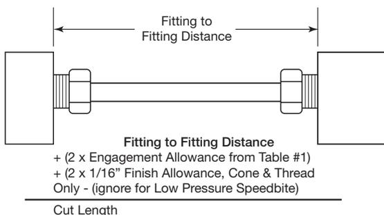
Fully annealed tubing (hardness max of 90 HRB) with proper outside diameter tolerances is recommended for these connection components.
