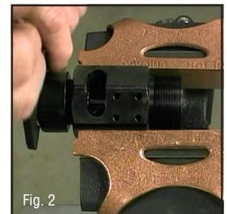
4. Slide the tubing through the collet until the end of the tube appears in the coning tool housing window (see Drawing in Table 3 above). Line the end of the tube with the edge of the window as marked above and tighten the collet nut firmly in place using the collet nut wrench (Fig. 2).
