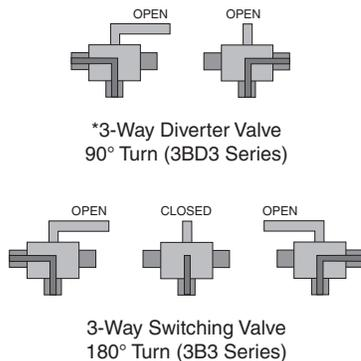
\*The Diverter Valve design permits inlet flow through the bottom port. Outlet flow may be diverted to either valve side port.
