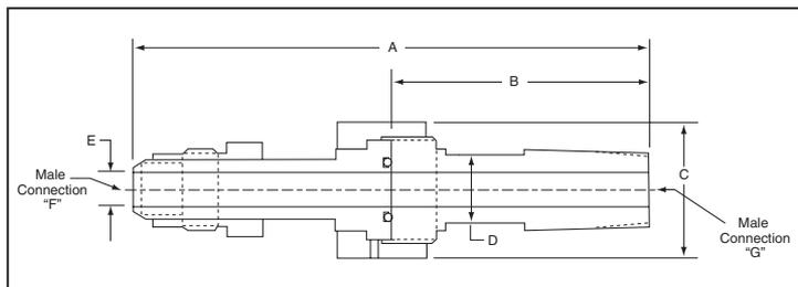
Note1: EZ-Unions are constructed from 316 SS and are supplied with a Viton o-ring as standard.
