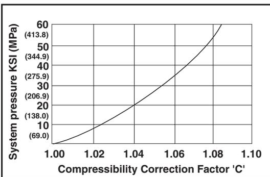
**Note:** Multiply pressure drop ( $\Delta P/\text{ft}$ ) from graph above by factor 'C' to correct for system pressure above atmospheric. Higher system pressure increases the fluid density resulting in higher system pressure loss.
