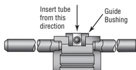
11. Apply pressure to the top of the threading tool to start the cutting action. The threads are left handed, so turn the threader **counterclockwise** to thread the tube.
