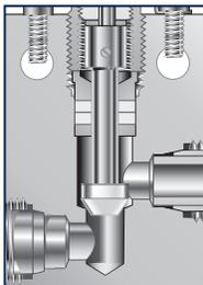
The Vee stem is used for direct on-off, metal-to-metal shut-off with quick-opening flow characteristics.
