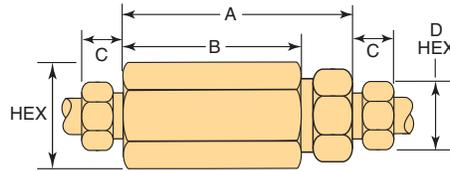
\*\* Larger micron size filter element is installed on upstream (inlet) side. All filters furnished complete with connection components unless otherwise specified.
