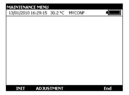
To adjust the T150, use the **ADJUST** function key. Make adjustments in the following order:
