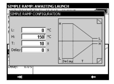
The parameters of a simple ramp are:
