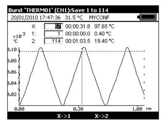
The left < and right > arrow buttons can be pressed to move the cursor and read off the abscissa and ordinate values. At this level, the markers can be redefined in order to zoom in between these two new points:
