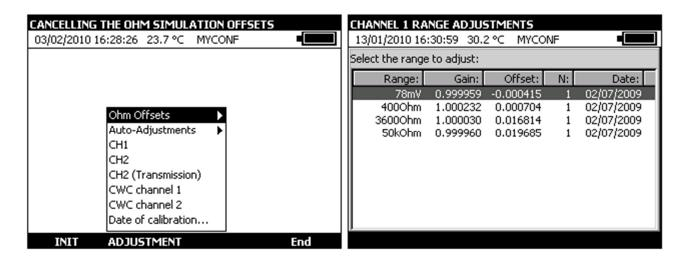
For each type of calibration, select the function to be calibrated with the Up  $\Lambda$  or Down V navigation keys and follow the instructions shown in the dialog boxes.
