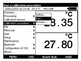
• To run a procedure, select it and press the **F4** key (Run) or **Enter** key.
