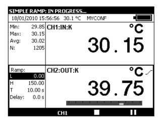
During generation of a simple ramp, a progress bar indicates the state of progress. The function keys are used to control generation:
