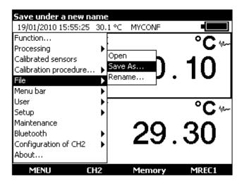
Use the navigation keys to select a configuration. Edit the name of the configuration to be saved with the alphanumeric keys and confirm with ENTER.
