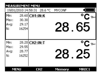
Two new functions, Memory and MREC1, then appear in the bottom bar (replacing the functions Rest stat. And Hold). The left < and right > arrow buttons can be used to switch from one mode to the other.
