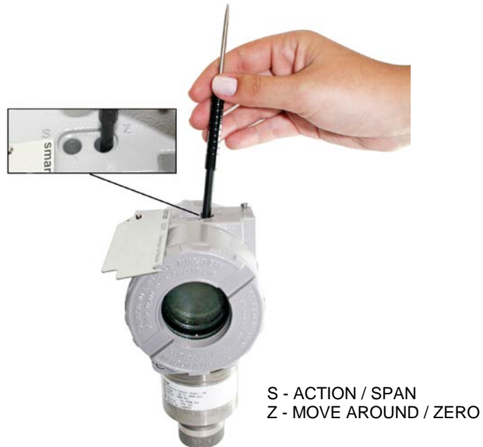
Figure 4.1 – Local Zero and Span Adjustment and Local Adjustment Switches
