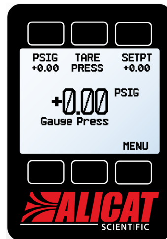
The main display . Note the button behind the logo, which toggles the device backlight.
