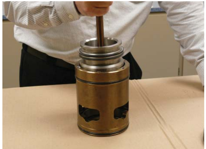
Figure 9-28 Install Shaft and Piston Assembly in Valve Cylinder
