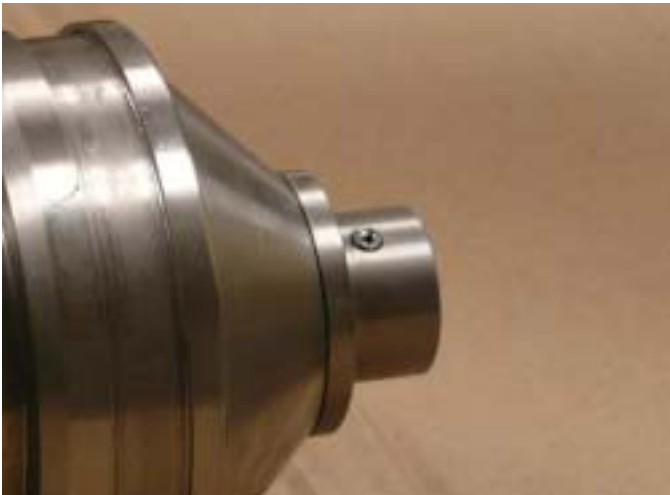
Figure 9-25 Press Spirol Pin
