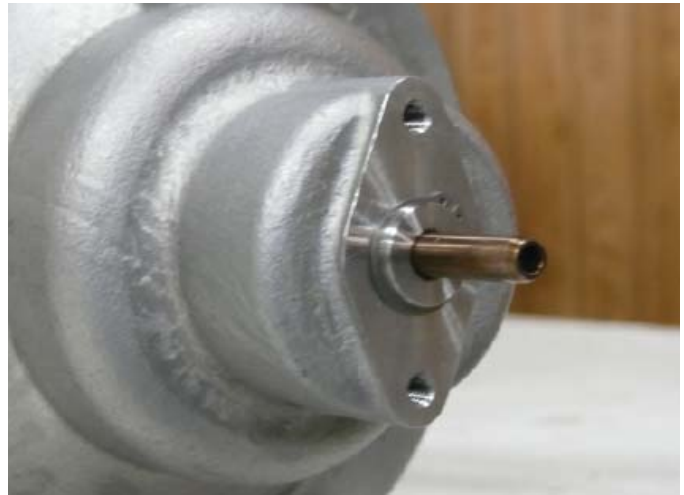
Figure 9-11 Remove Retaining Ring
