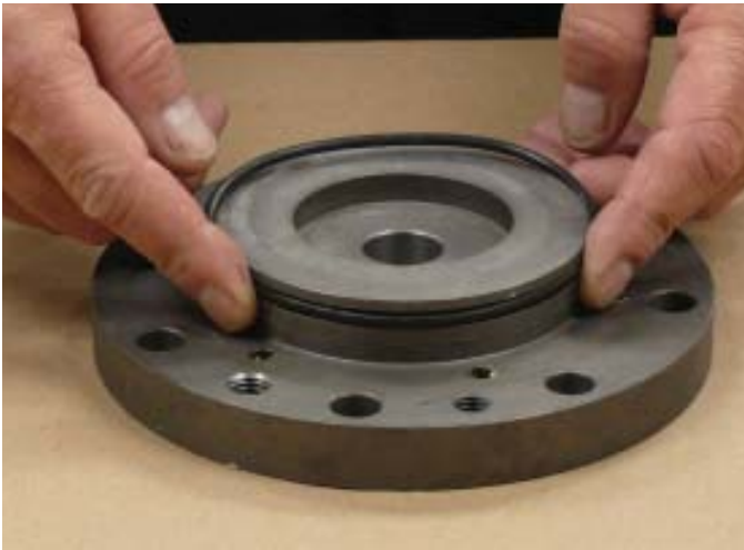
Figure 9-30 Install O-ring on Cylinder Head
