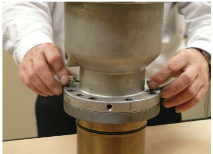
Figure 9-32 Install Motor Housing
