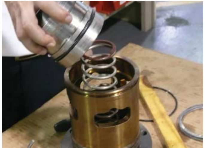
Figure 9-8 Removing Spring From Cylinder
