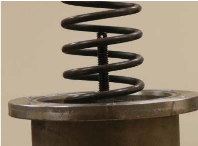
Figure 9-36 Install Spring in Housing
