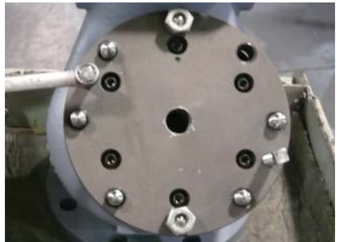
Figure 9-1 Alternately Tighten Jack Screw
