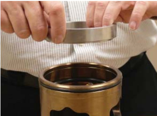
Figure 9-26 Install Seal Ring
