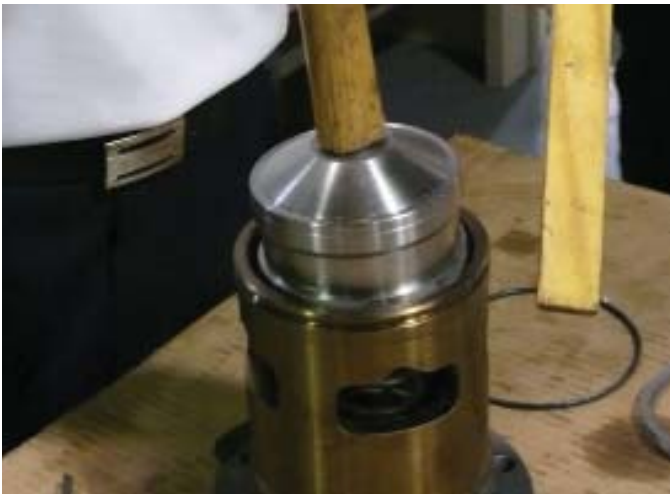
Figure 9-7 Removing Spring From Cylinder
