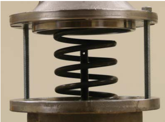
Figure 9-37 Thread Hex Head Bolts into Motor Housing
