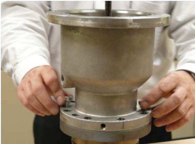
Figure 9-12 Remove Power Cylinder Assembly from Main Valve Body
