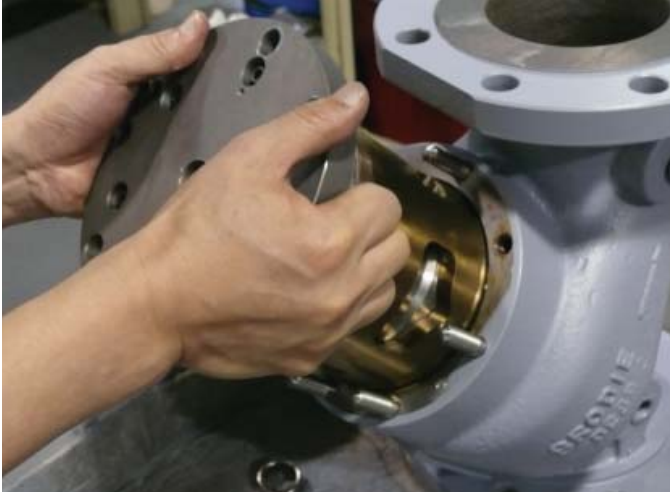
Figure 9-2 Remove Cylinder Assembly From Valve Body
