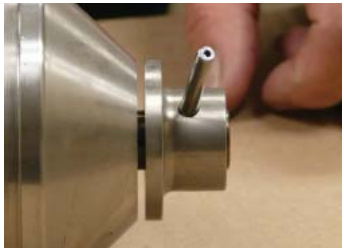
Figure 9-24 Press Spirol Pin
