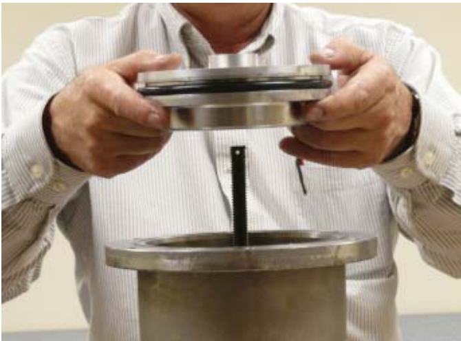
Figure 9-34 Install Motor Piston over Shaft
