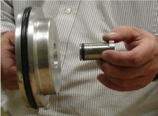
Figure 9-33 Install Motor Piston Bushing
