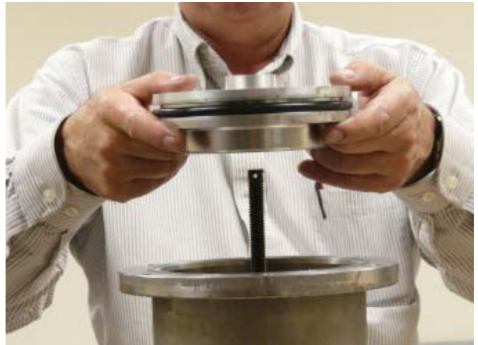
Figure 9-14 Remove Piston from Power Cylinder Assembly
