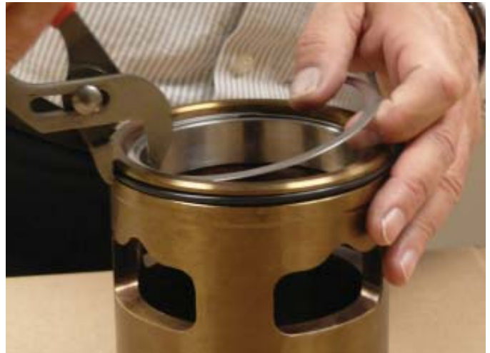
Figure 9-27 Install Retaining Ring
