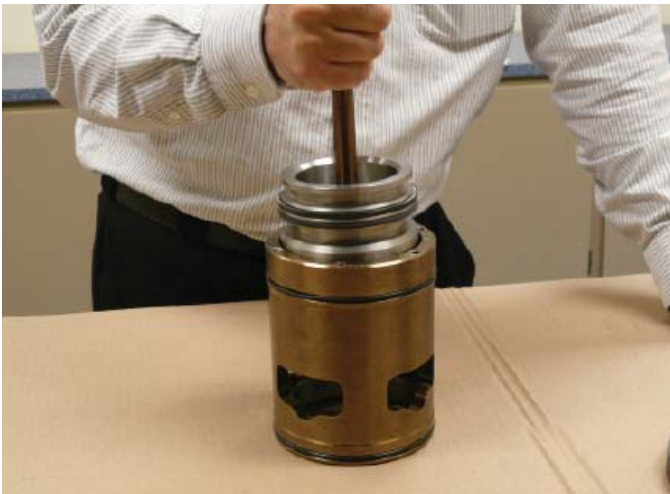
Figure 9-16 Remove Piston and Shaft Assembly
