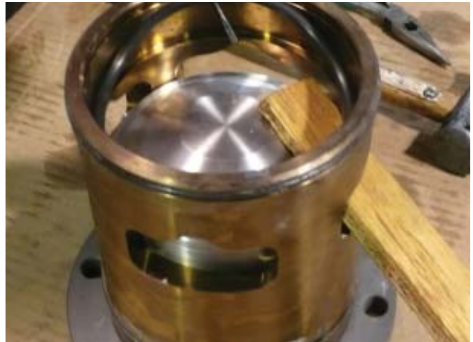
Figure 9-3 Block Piston In Open Position
