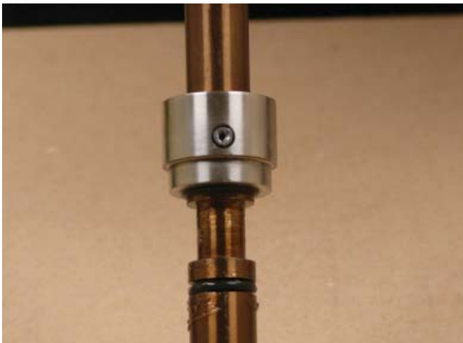
Figure 9-18 O-ring Sleeve and Spirol Pin
