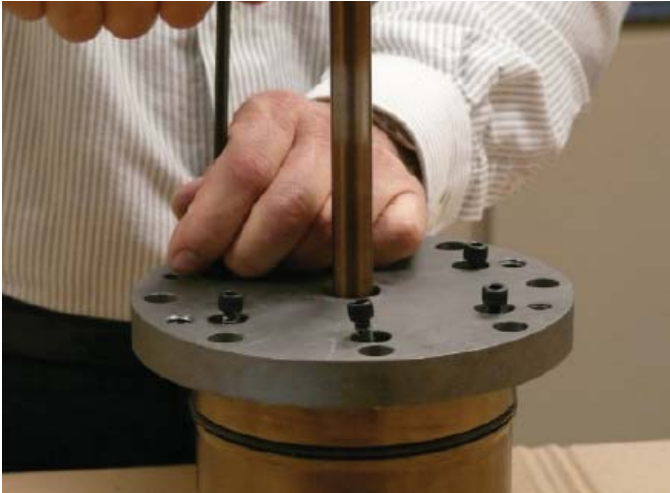
Figure 9-15 Separate Valve Cylinder from Cylinder Head
