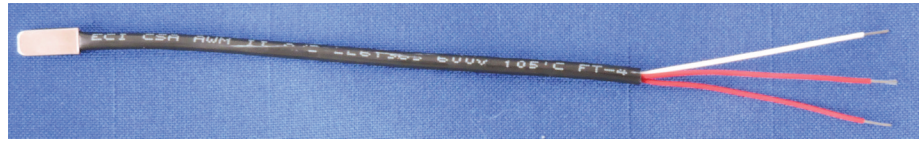
Fig 2. R342 with Single 3-wire RTD shown
